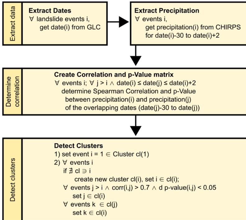
Figure S1. Flowchart of the algorithm to detect clusters within the global landslide catalog (GLC). Symbols included:  $\forall$  - for all;  $\wedge$  - logical conjunction;  $\in$  - element of;  $\nexists$  - there does not exist;  $\ni$  - contains.
