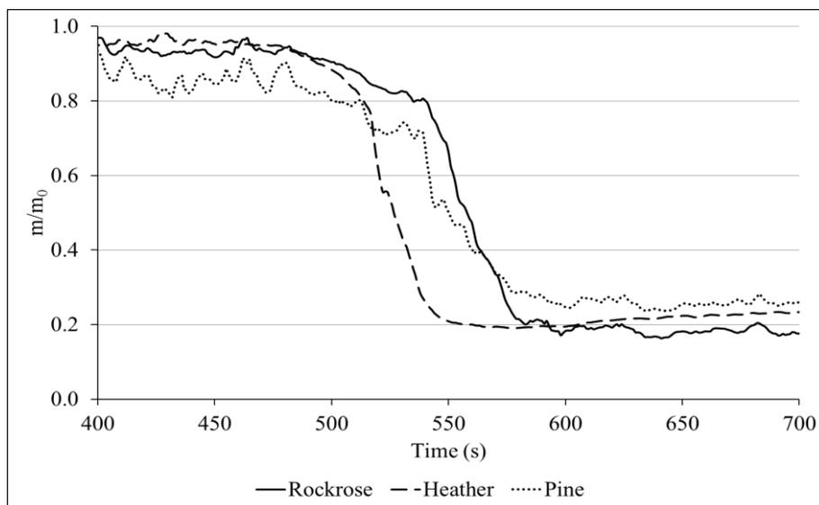
Figure 6: Experimental mass losses obtained at field scale.
