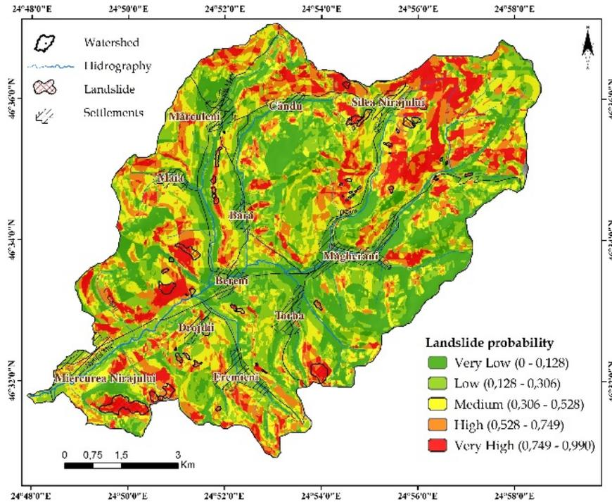
Figure 3. Landslide susceptibility map generated using the logistic model.
