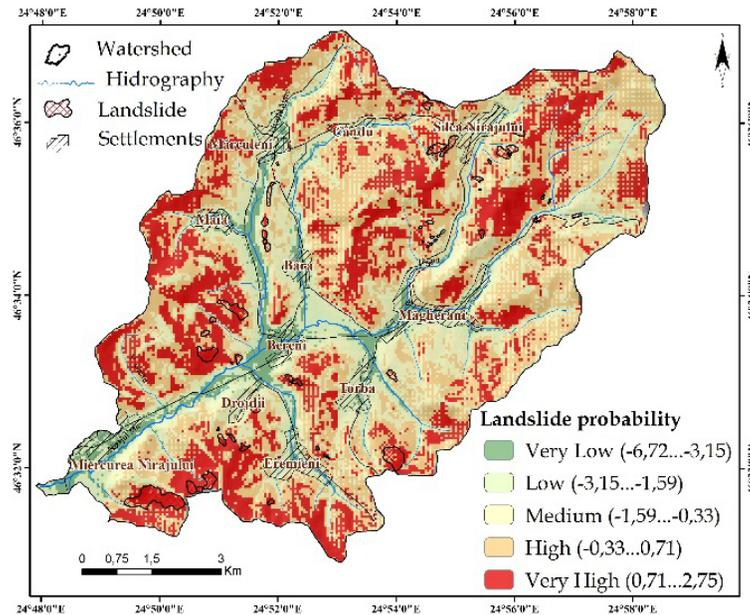
**Figure 5.** Landslide susceptibility map generated using the BSA model.
