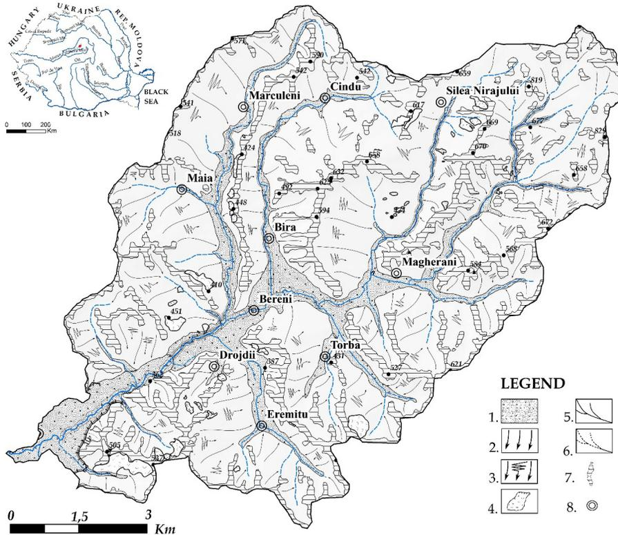
**Figure 1.** Geomorphological map of the Small Niraj catchment and geographical position of the study area (1 – flood plain, 2 – slopes and connecting surfaces, 3 – slopes with complex modelation, 4 – active landslides, 5 – permanent hydrographic network, 6 – temporary hydrographic network, 7 – watershed divide, 8 – settlements).
