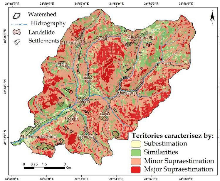
**Figure 7.** Regional differences of susceptibility classes obtained through BSA model or by applying logistic model.
