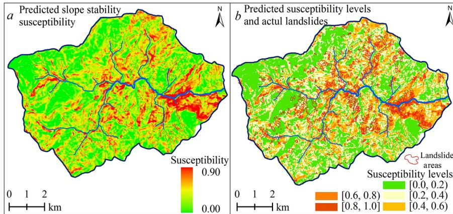
**Figure 6.** Predicted slope stability (a) and the susceptibility levels (b) in the Subao River basin.
