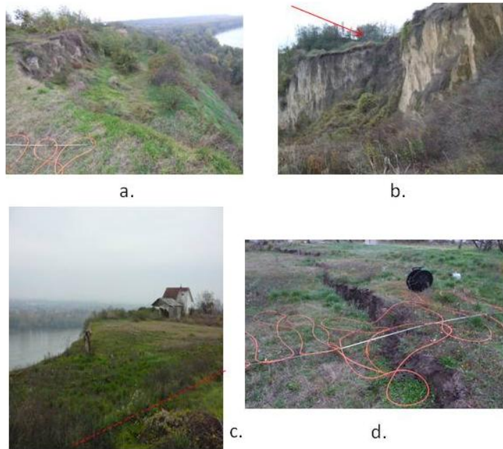
Figure 3. (a) The rock mass which has already been slipped looking from South, from the study area. (b) The quasi vertical wall along the collapse. The arrow indicates the research area. (c) The study area from western direction with tapes along many profiles and with river Danube in the background. The profiles are closely west–east orientated. The red dotted line shows the main fracture which can be directly seen from the opposite direction. The wall is in about 6 m distance from the East end of the tapes. (d) The main fracture from East direction with profiles S4–10. The main crack branches off here. In the background the area which have been cultivated. The long profile (P2) elongated between the two wine yards in line S10.
